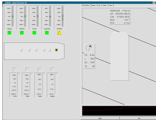
Figure 3: GUI presenting real-time loads on the hull, alarms and sea state parameters
